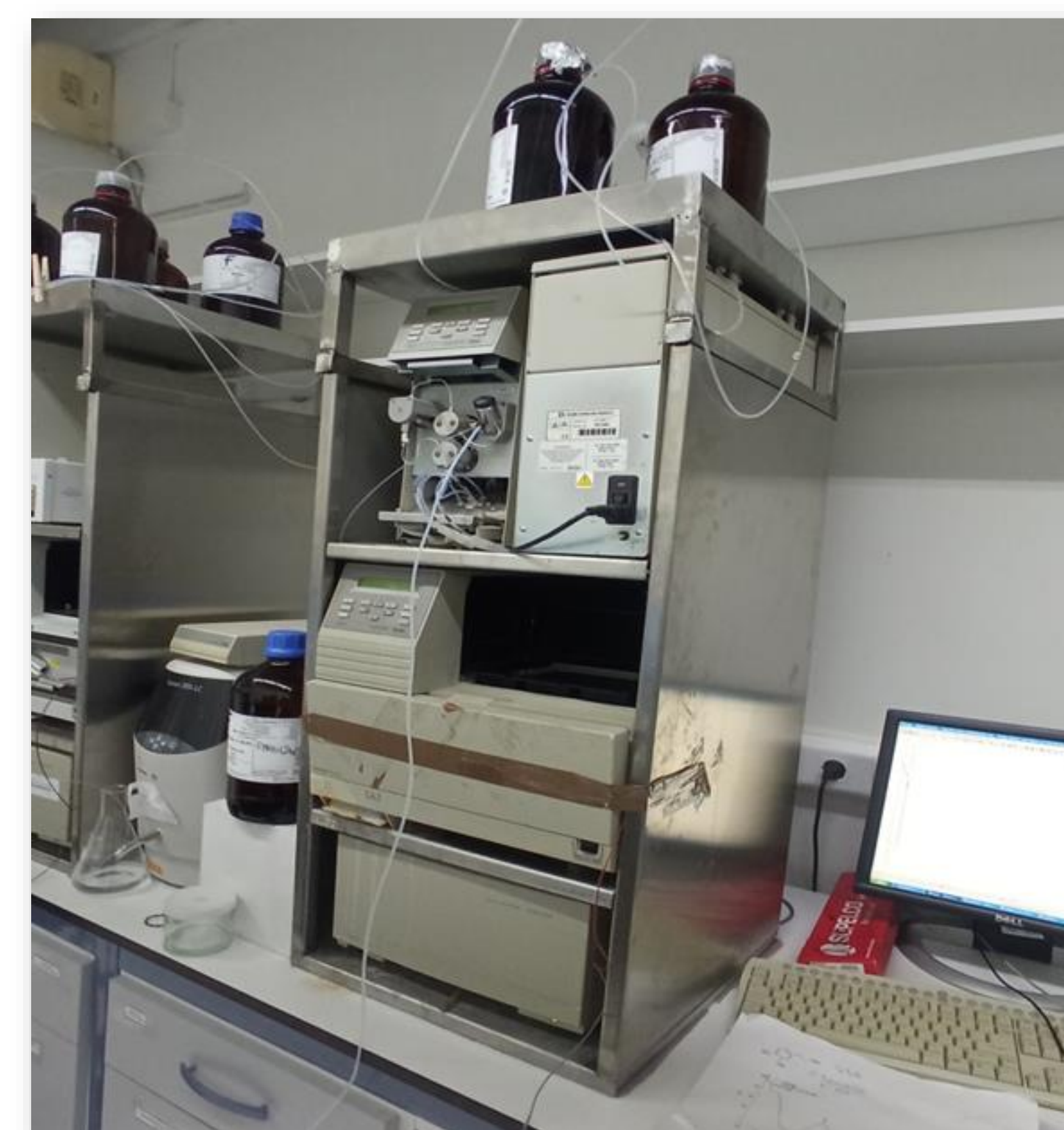
Figure 1: HPLC equipment used for separation and quantification of biophenols in olive oil in Pharmacognosy & Natural Products Chemistry/ University National of Athene.
